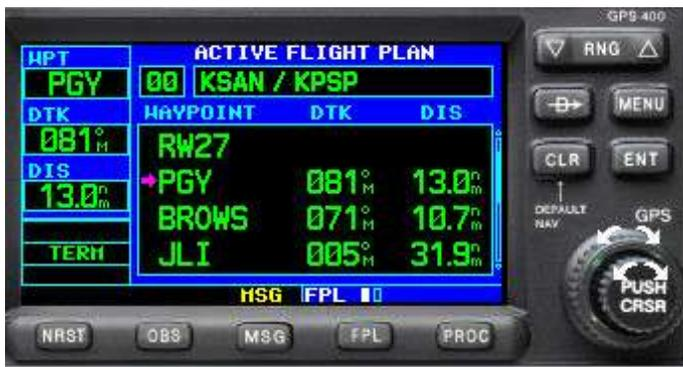
The ACTIVE FLIGHT PLAN shows that a SID has been loaded, for a runway 27 departure, JLI transition.
