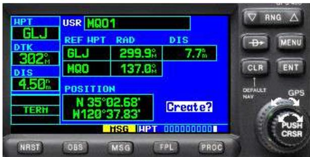
Enter **300.0** in the **RAD** box. (NOTE: The Garmin may change your entry by 1/10<sup>th</sup> of a degree. That's acceptable). Press **ENT**, which advances the cursor to the **DIS** box. Accept the value (do not modify it) by pressing **ENT**.
