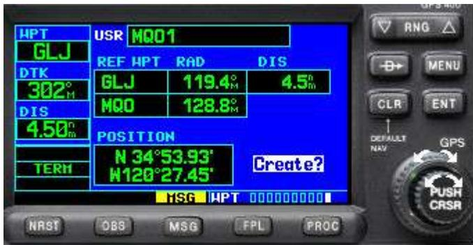
**Create?** is highlighted (the cursor starts there), but you don't want to create it yet. Using the large knob, move the cursor and highlight the top **REF WPT** box. If GLJ is not there, use the small and large knobs to enter it. From this point, the cursor is advanced to **RAD** by pressing **ENT**.
