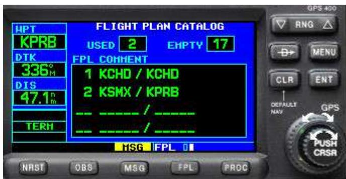
Activate the cursor and highlight the desired Flight Plan (#2),
