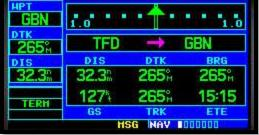
Alternately, you can press and hold the CLR button, and from any section or page, it will take you to the DEFAULT NAV page. Then, using the small knob, turn it clockwise to the end (page 6)
