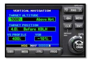
Press the small knob to activate the cursor. This highlights the ALTITUDE value. You can change it using the small and LARGE knobs. In this case, we have entered 1000 feet.
