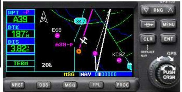
As you approach the end of the flight plan, a message will annunciate PTK END
