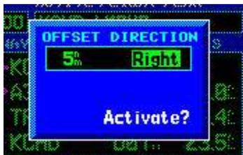
Using the small knob, select the number of miles. Press **ENT** and select "Right" or "Left", then **ENT**. Then press **Activate?**
