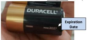
In plain English, all of the batteries must have the same expiration date and they must be replaced upon reaching 50% of their useful life, based on the expiration date on each battery cell.
