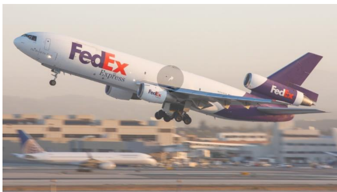
This MD10 had undergone a major transformation and now not only possessed new glass cockpit technology, but it also only required two crewmembers to fly.
