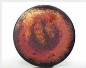
Don't be alarmed by the bright color, or deposits around the edges. The symmetrical pattern shows this valve is just fine.
