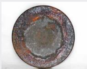
A symmetrical, circular pattern shows a healthy valve. Red and orange deposits are harmless.
