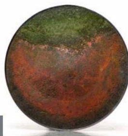
5 Green crescent progresses toward center with valve cracking and failure a serious danger.
