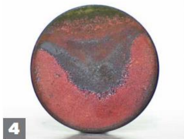
4 GREEN MEANS STOP. The green area at the top shows this valve should be replaced immediately. (Note how the uneven burn patterns match the heat distribution chart.)
