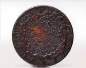
Thick lead deposits from an overly rich mixture give this healthy valve the appearance of an overcooked pizza.
