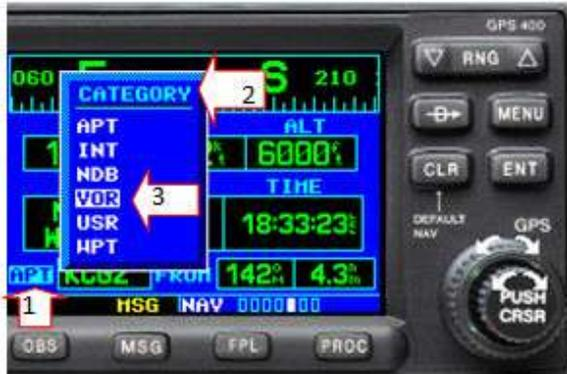
Using the large knob, move the cursor on the page until “APT” (arrow #1) is highlighted.
