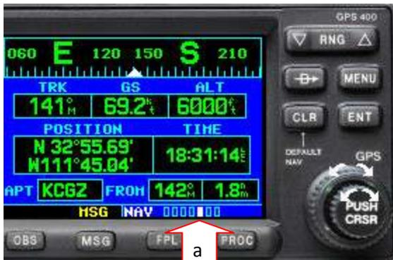
While in the NAV chapter . . . turn the small knob clockwise to **NAV 5** (shown by arrow “a”) – or just turn the small knob all the way to the end of the NAV chapter (Vertical Nav page or NAV 7). Then, click counter clockwise two clicks to NAV 5.
