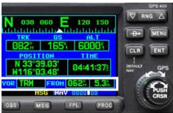
Next time that you want to call ATC out of the blue for flight following and you’re in the middle of nowhere, just go to page 5 of the NAV chapter. The “POSITION” Page will be all set up for the closest VOR and Radial/DME. Now that’s service! In this case, you’re on the Thermal VOR (TRM) 062° radial at 5.3 nm.
