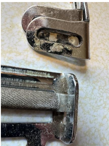
Corroded belt hardware
