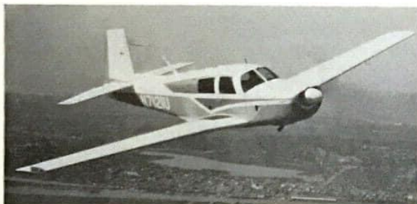
MOONEY SUPER 21 — The convincing new Super 21 with Positive Control. 200hp with 187mph cruise. Ram air power boost adds another 10-12hp at altitude.
