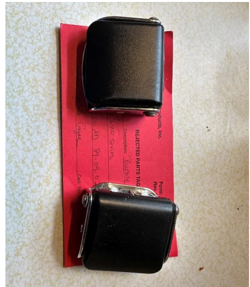
Original buckles red tagged due to AD
