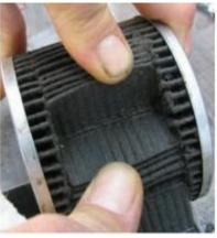
The first place is in the "Suction Screen" that sits close to your oil pan. This catches the relatively large pieces of metal (.03" or larger) and prevents it from traveling any further into your engine.
